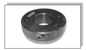
The actuator screws has to be turned into the body by using the enclosed Allen key. The internal medium will flow into the circulargroove and raise the ring piston. With less manual force you create a big hydraulic clamping force. For to relieve the clamp nut put the actuator screws to the start position and move the nut to the opposite direction. The medium remains into the system.
