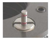
Pressure indicator is designed for easy presentation of existing system pressure within clamp nut. On the basis of the marks at pressure indicator clamp force can be derived from.
