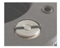
Picture shows pressure indicator visible up to 1. mark.
