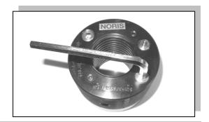
The actuator screws has to be turned into the body by using the enclosed Allen key.
