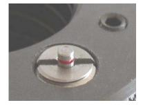
Picture shows pressure indicator visible up to 2. mark.
