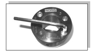
The actuator screws has to be turned into the body by using the enclosed Allen key. The internal medium will flow into the circulargroove and raise the ring piston. With less manual force you create a big hydraulic clamping force. For to relieve the clamp nut put the actuator screws to the start position and move the nut to the opposite direction. The medium remains into the system.
